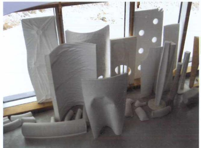
of formwork and geotextile required in the build process, and finally the design approach. Responding to requirements for material efficiency, improved integral strength and adapting established formwork techniques to produce larger scale span structures, new ideas for in-filled formwork through the use of load-bearing textile reinforcement evolved.
