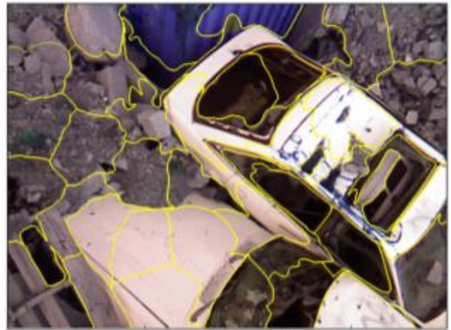
Figure 2. SLIC superpixel segmentation of RGB image using an initial number of 50 superpixels.
