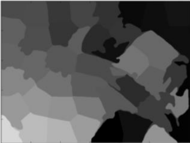
Figure 5. SLIC superpixel segmentation of depth image with average RGB values within each of the 50 superpixel regions computed.
