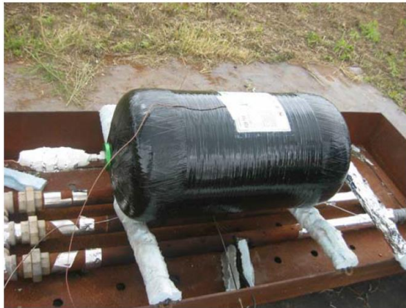
Figure 7.1 Hydrogen fuel tank test setup (Zalosh, 2007)
