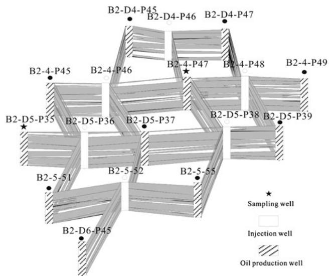
**Fig. 1** Five-spot well patterns applied in six injection wells and 11 production wells in the studied block of Daqing Oil Field (China). The white parts between wells represent the continuity of the studied reservoir
