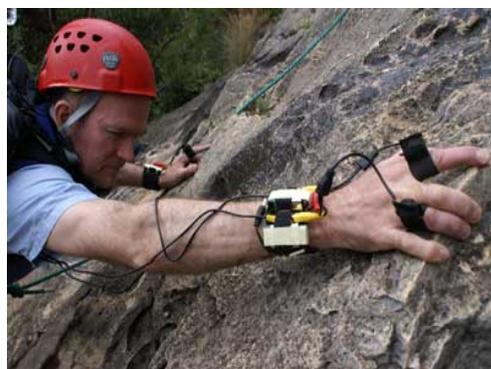
We now have a lightweight system where John can wear tiny adapted cameras on his fingers and climbing shoes as well as higher grade cameras attached to his backpack. In total we have eight unobtrusive onboard cameras recording his climbing activity. This equipment is being tested and used in a variety of locations.
