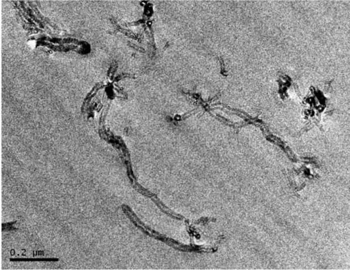
Figure 8. TEM image of the nitric functionalized CNT dispersed in THF (individual CNTs observed).
