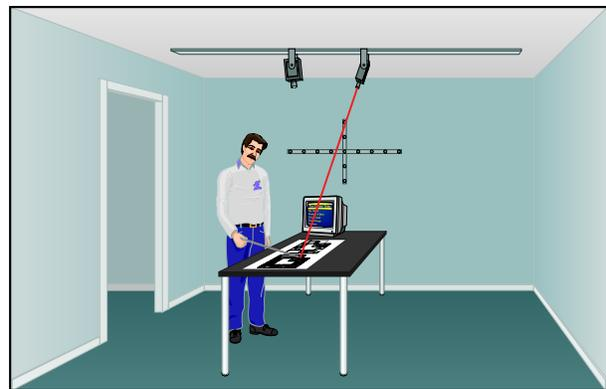
Figure 2: Physical layout of the IntelliMedia Work-Bench
