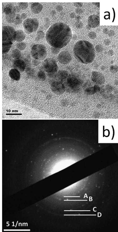
**Fig. 3** (a) Transmission electron microscopy (TEM) image of SiSn nanocrystals produced by ns pulsed laser ablation in water of a SiSn target. (b) Corresponding diffraction pattern showing spots arranged in four concentric rings around a central very bright spot, marked by A, B, C, D.
