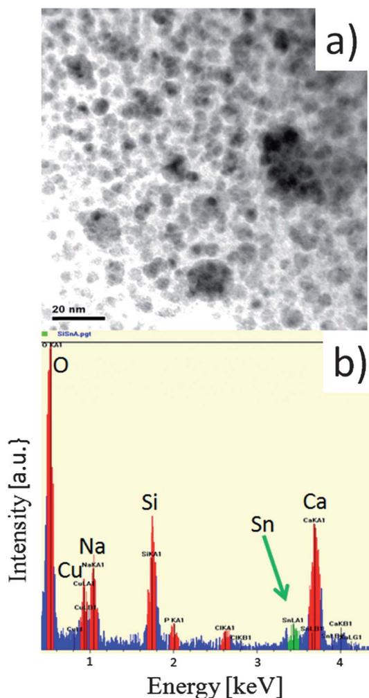
**Fig. 1** (a) Transmission electron microscopy (TEM) image of SiSn nanocrystals produced by pulsed ns laser ablation in water of SiSn targets and dispersed on a TEM grid. (b) Corresponding energy-dispersive X-ray spectrum.
