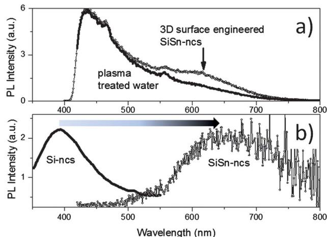
**Fig. 4** (a) Photoluminescence (PL) spectra of the SiSn nanocrystal (SiSn-NC)–water colloid as-prepared by ns laser processing (full line) and after microplasma surface engineering for 32 minutes (open symbols/full line); excitation at 400 nm. (b) PL spectrum (400 nm excitation) of the SiSn-NCs after extraction of the background (open symbols/full line) and, for comparison, typical PL spectrum of elemental Si-NCs prepared by ns laser ablation in water and excited with wavelength at 300 nm.
