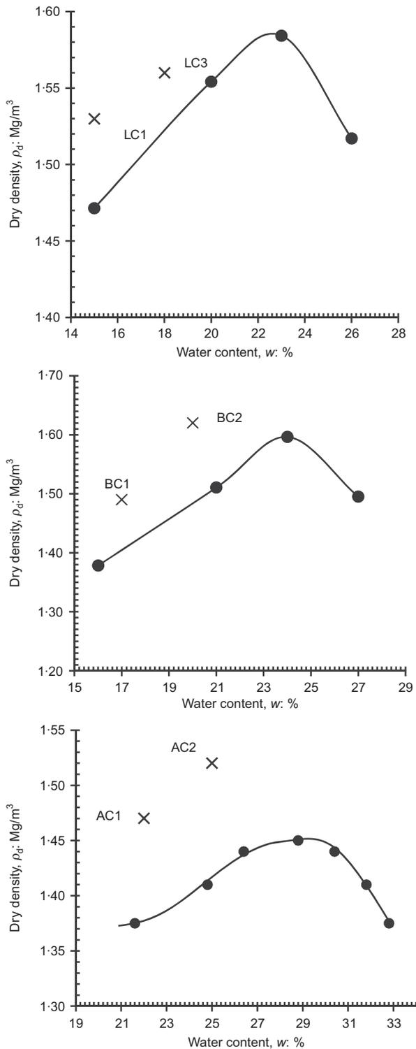
Fig. 3. Proctor compaction: London Clay, Belfast Clay and Amthill Clay
