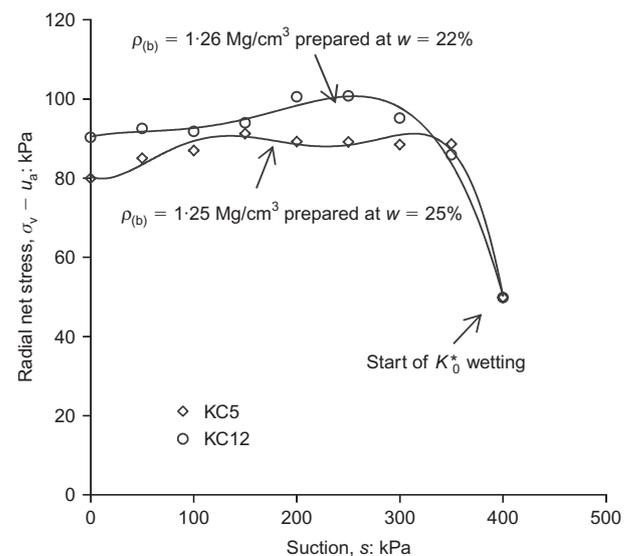
**Fig. 8.** Effect of compaction water content for a given initial dry density
