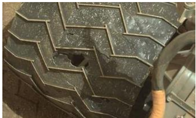
Figure 5. Curiosity wheel damage – many cracks like this have been found on all six wheels of the rover [13].
