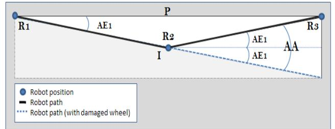
(a) Robot error correction using 1 interval
