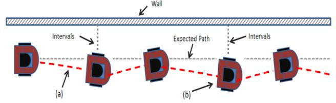
Figure 11. Shows the path of the Pioneer P3-DX robot when it implements the compensation algorithm. (a) Wheel damage causes the robot to ‘slew’ away from the expected path. (b) When the robot reaches an interval point, the robot is stopped and then turned on its axis at the required angle for adjustment..
