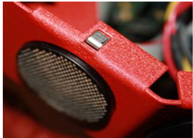
Figure 4. Polaroid Sonar Sensor Transducer is used for operations in air at ultrasonic frequencies.
