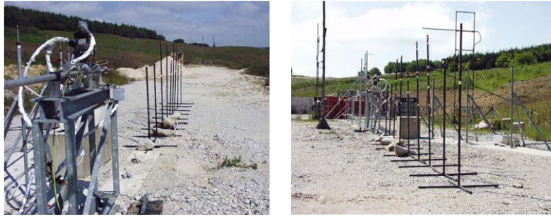
Figure 1. Experiment layout: view from the release nozzle to oxygen depletion sensors (left); view from oxygen depletion sensors towards the release nozzle (right) [11]
