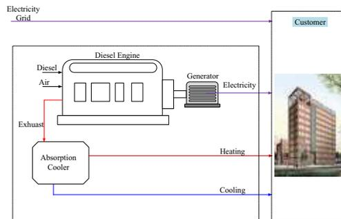
Fig. 1. A typical DG system
