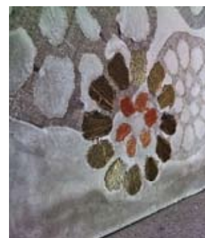
Girli Concrete produces panels by placing textile (cashmere, flocked fabric and even lace from Northern Ireland) in a mould with cement poured over and left to dry over a period of almost a whole month. The material has an intriguing visual and tactile aesthetic, but has the possibility to provide acoustic insulation as well. www.ulster.ac.uk
