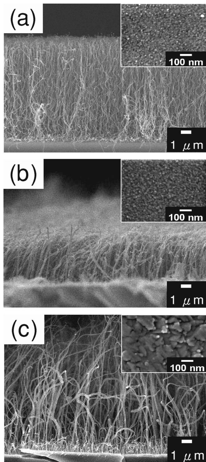
**Figure 1.** Cross-sectional SEM images of  $\text{CN}_x$  NTs on (a) bare Si, (b) Ti (20 nm)/Si, and (c) Ti (200 nm)/Si substrates. The insets are plan-view SEM images of the catalyst layer after a  $\text{H}_2$  plasma treatment.
