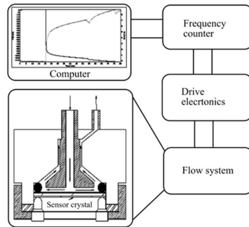
Fig. 1 A schematic illustration of the QCM-D system.
