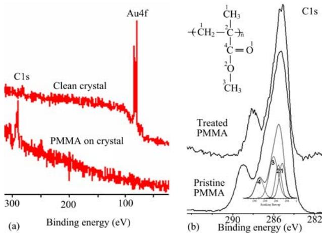
**Fig. 2** (a) XPS spectrum for clean crystal surface and PMMA spin coated crystal surface; (b) C1s XPS spectra of the pristine and DBD processed PMMA surface with fitted peaks associated to the repeating structural units of the polymer.
