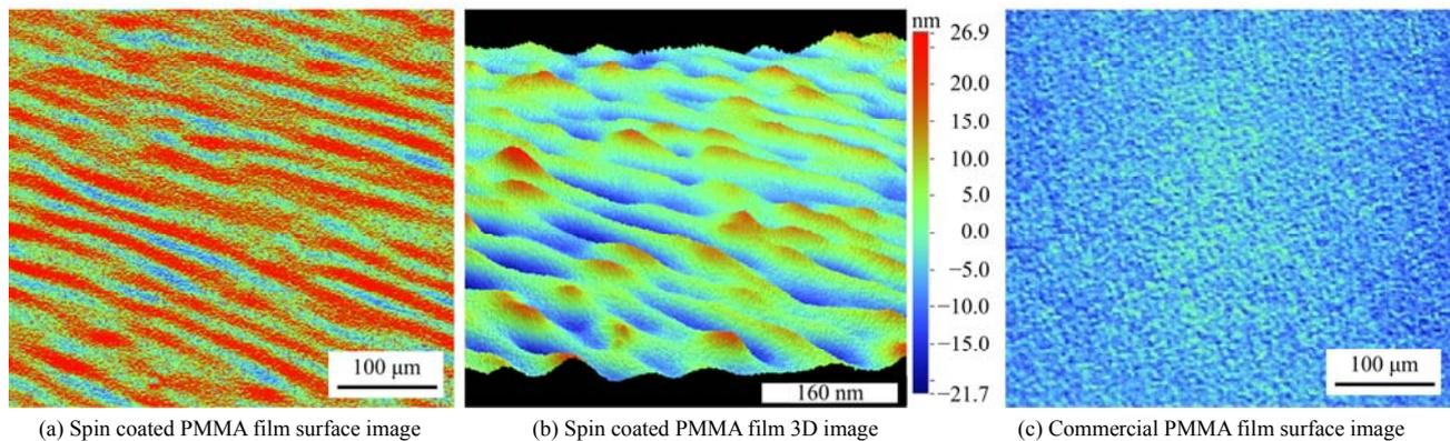
Fig. 8 Surface optical profilometry images.
