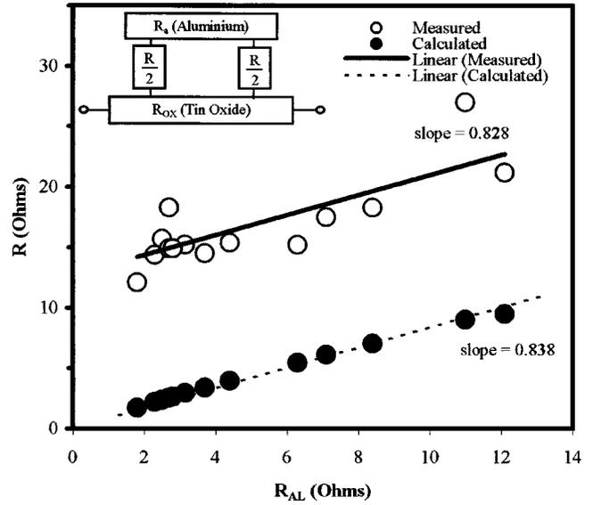
FIG. 3. Experimental and calculated resistance of the combined tin oxide-aluminum electrode. A lumped contact resistance ( $R/2$  in the inset model) of  $7.5 \Omega$  yields the solid line drawn through the experimental data.
