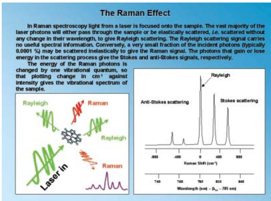
so is filtered out of the signal. In addition to the Rayleigh scattering, Raman scattering, in which the frequency of the incident photons changes due to interaction with the sample, can also be detected. Unfortunately, the Raman scattering comprises a very small fraction of the incident photons, typically 0.0001 %, hence the need for an intense source and sensitive detector.
