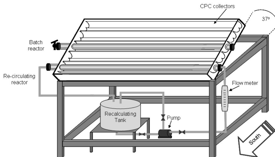
Figure 1: Schematic batch and re-circulating solar photoreactor.
