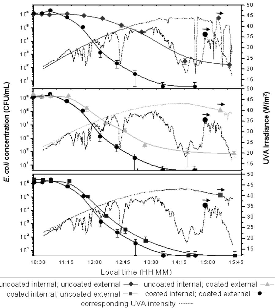
Figure 4: Solar photocatalytic disinfection in 7 L re-circulating reactor.
