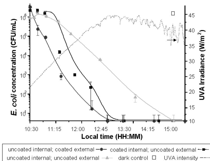
Figure 2: Solar photocatalytic disinfection in 1.25 L batch reactor.
