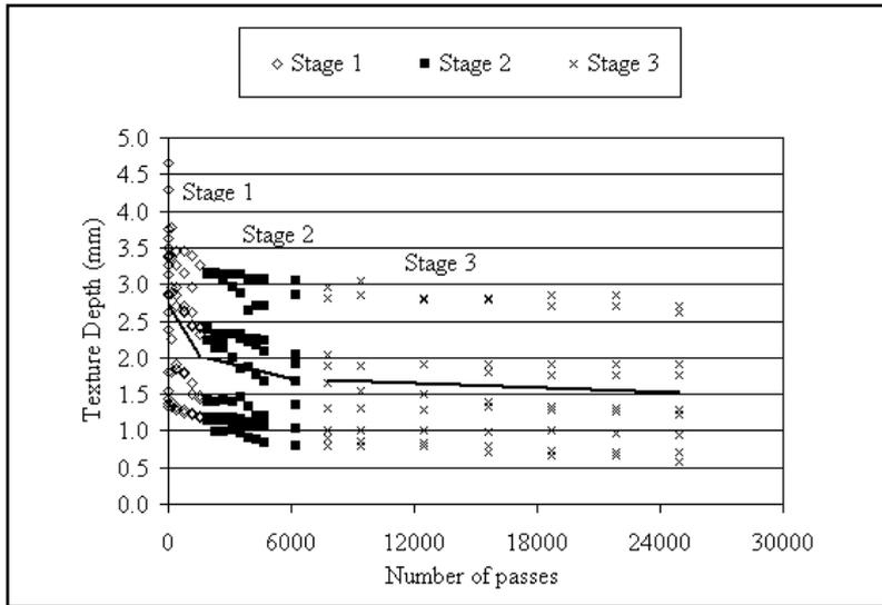
Figure 4: Three stages of texture depth change
