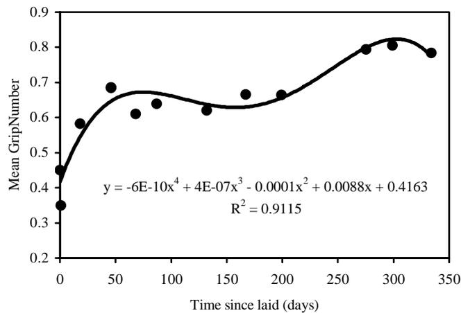
Figure 4 Change in GripNumber with time for a section of 14mm SMA
