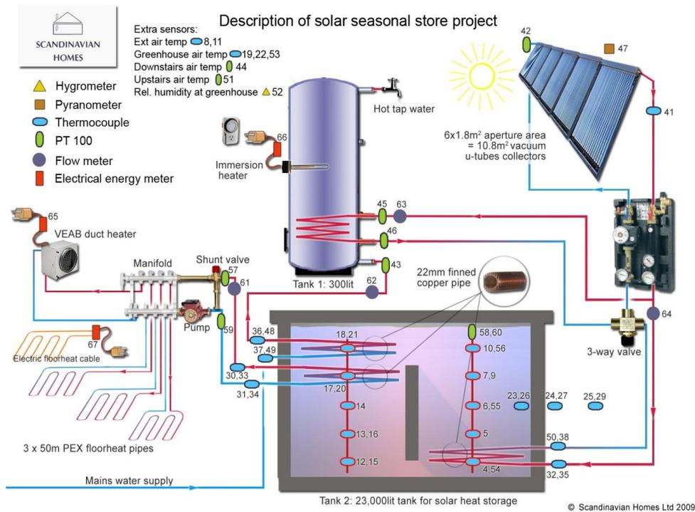
**Fig 1. Diagram of monitored Solar Installation**
