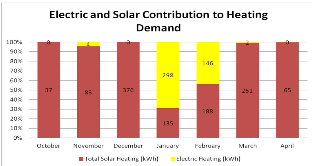
**Fig 2 Space Heating Demand for Oct 2010 to Apr 2011 with Solar Fraction per Month**
