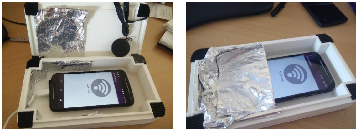
Figure 2. A proof of concept listener to evaluate the viability of electromagnetic shielding to provide a beamformed egress detection zone.
