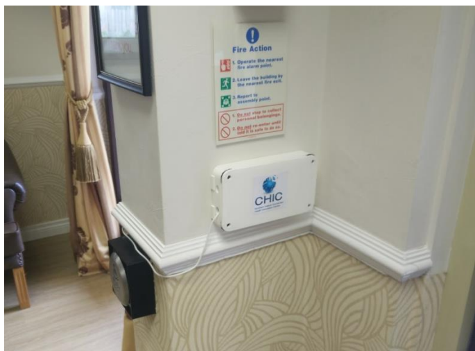
Figure 8. The deployment of the solution within a residential care home. This was subsequently used to monitor unsafe egress of a number of residents.
