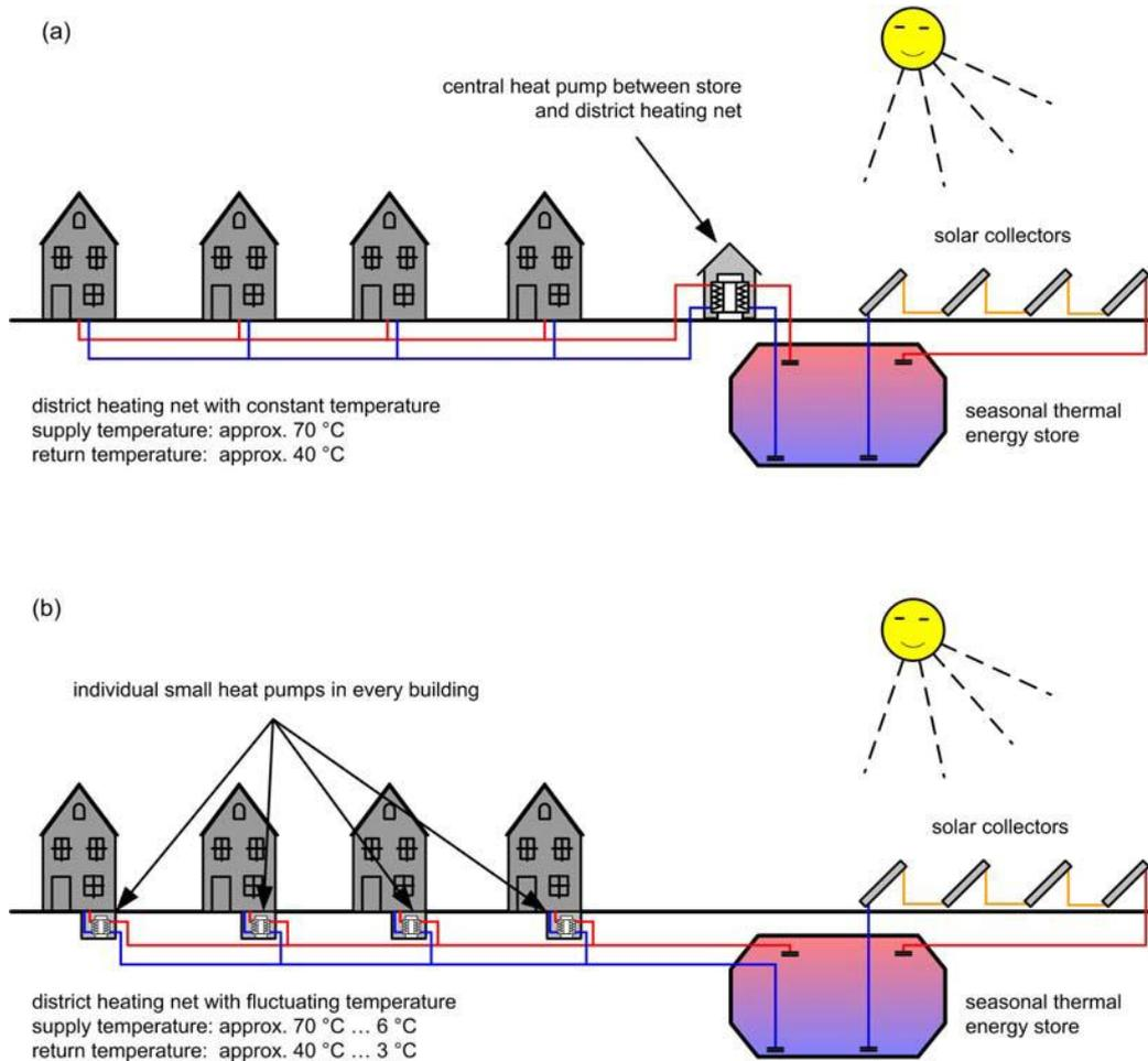
Figure 1 (a) Central heat pump (b) distributed heat pump, in combination with STES
