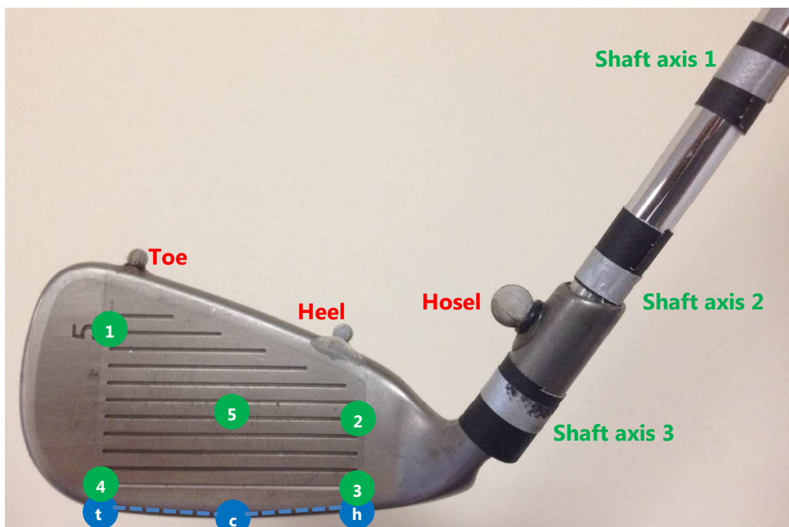
Figure 2: Marker placement on clubhead and hosel.
