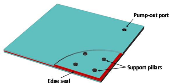
Fig. 1 A schematic diagram of VG
