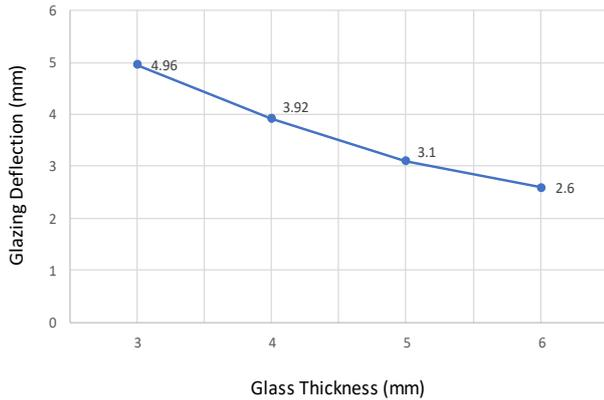
Fig. 4 VG deflection for different glass thicknesses
