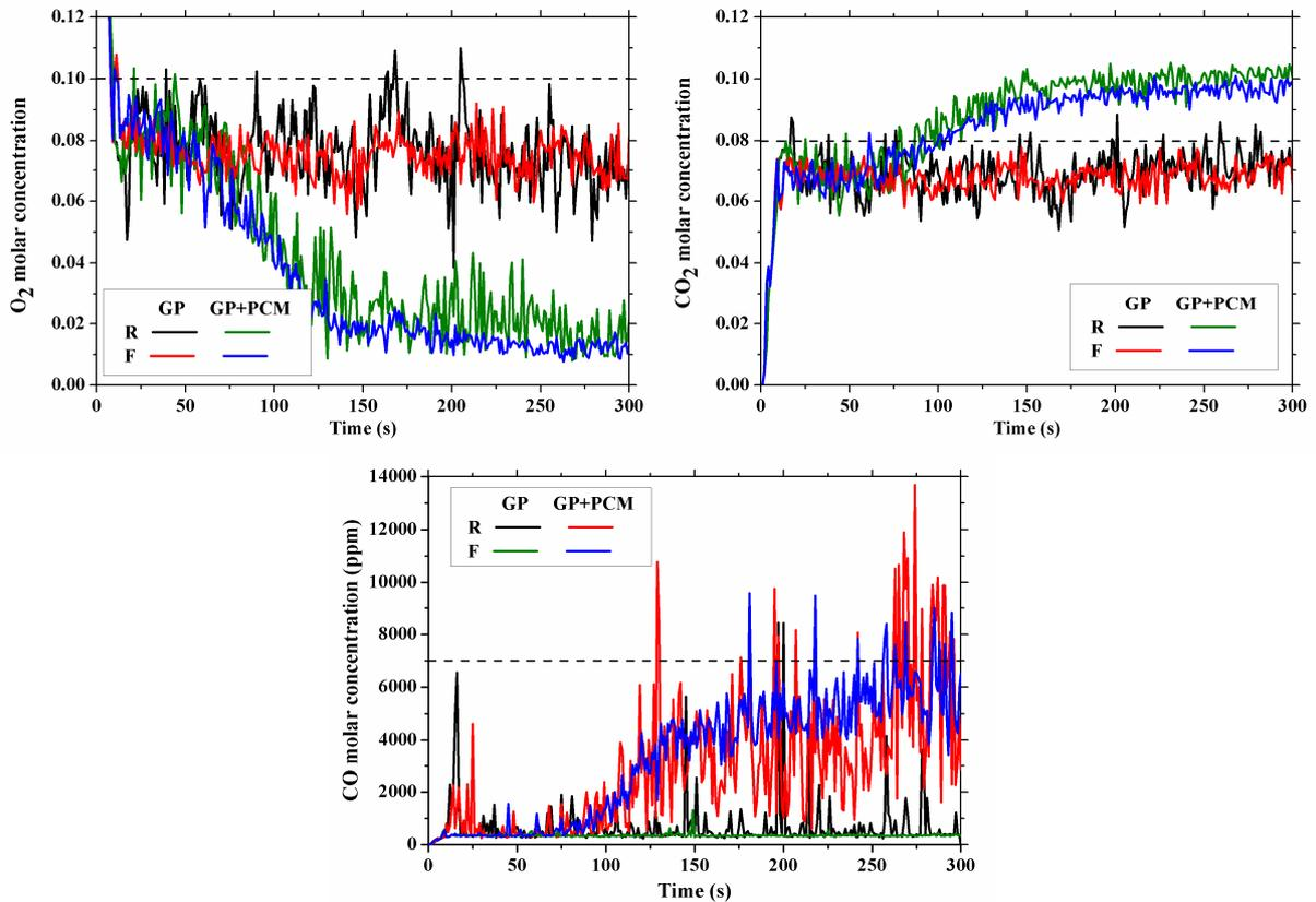
Figure 10. Temporal evolution of O<sub>2</sub> (top left), CO<sub>2</sub> (top right) and CO (bottom) molar concentrations at a height of 2.0 m.
