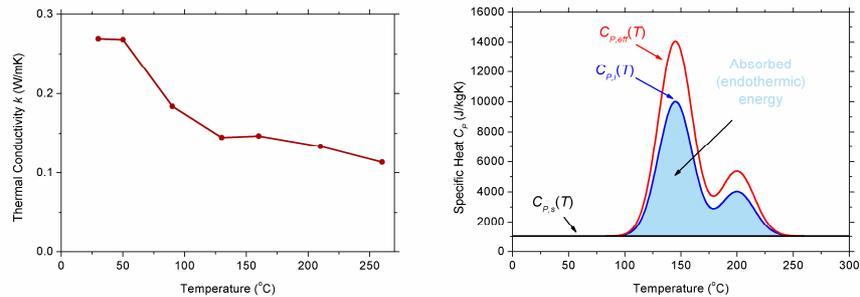
Figure 3. Temperature dependent thermo-physical properties of gypsum plasterboard.
