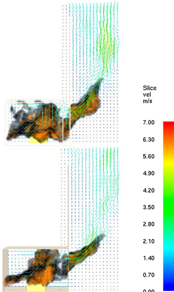
**Figure 10:** Predictions of velocity vectors and flame envelope for Test Case 1 (top), 525 s after fire initiation, and 2 (bottom), 595 s after fire initiation.
