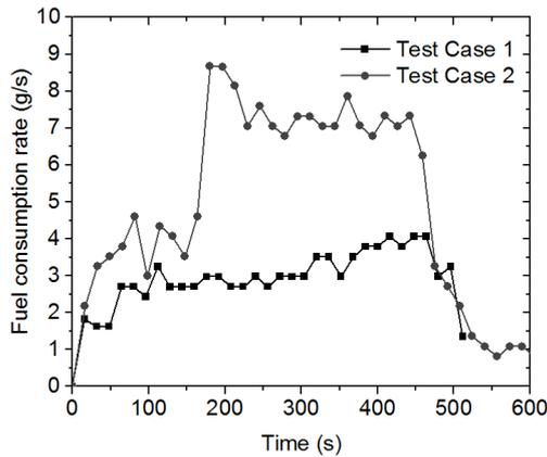
Figure 2: Measurements of instantaneous fuel consumption rate for Test Cases 1 and 2.
