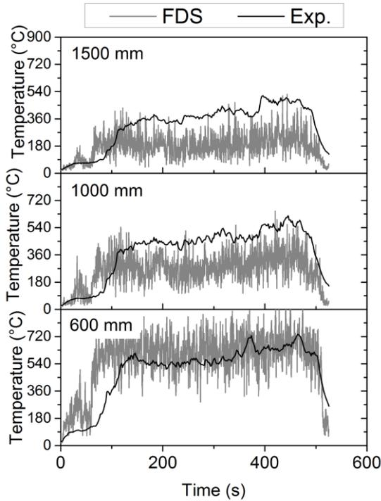
**Figure 5:** Temperature histories at a height of 600 mm, 1000 mm and 1500, 123 mm (location TC1) from the façade (Test Case 1).
