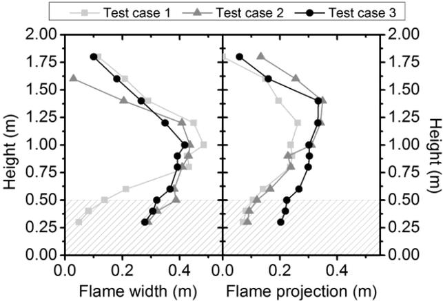
**Figure 10.** Vertical distribution of the time averaged flame width and projection.
