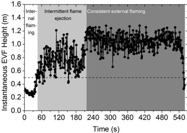
**Figure 8.** Temporal evolution of instantaneous flame height for Test case 3.
