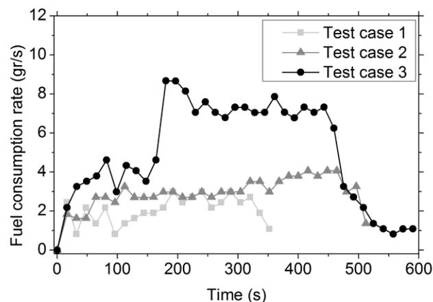
**Figure 3.** Measurements of instantaneous fuel mass consumption rate.
