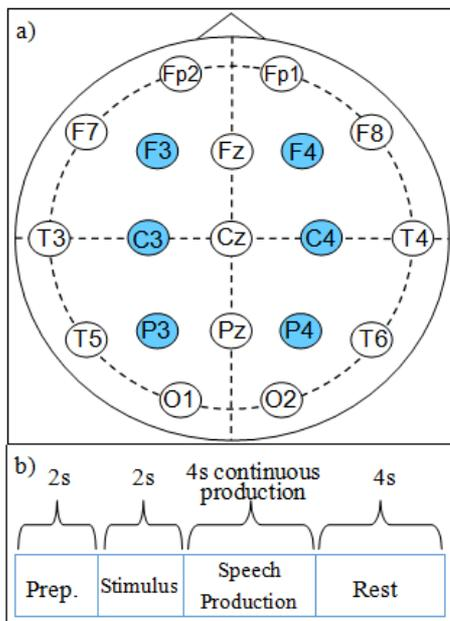
Figure 1 a) 6-electrode montage. b) Experimental protocol.
