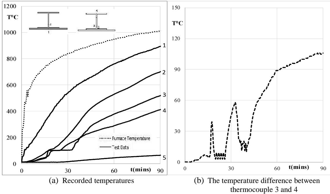
Fig 2: Recorded test data for the slim floor beam assembly with web openings
