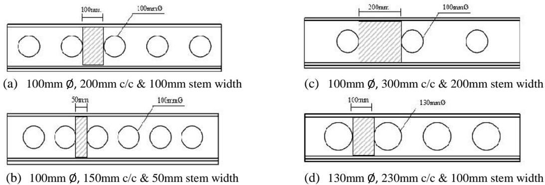
Fig 4: Sensitivity study, the effect of the spacing and size of openings
