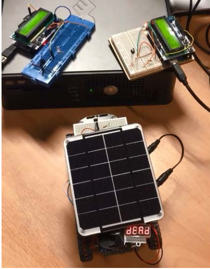
Figure 7 “ dead ”; A damaged sat that has lost its right to operate and has had its apoptotic mechanism triggered (pre-programmed self-destruct)
