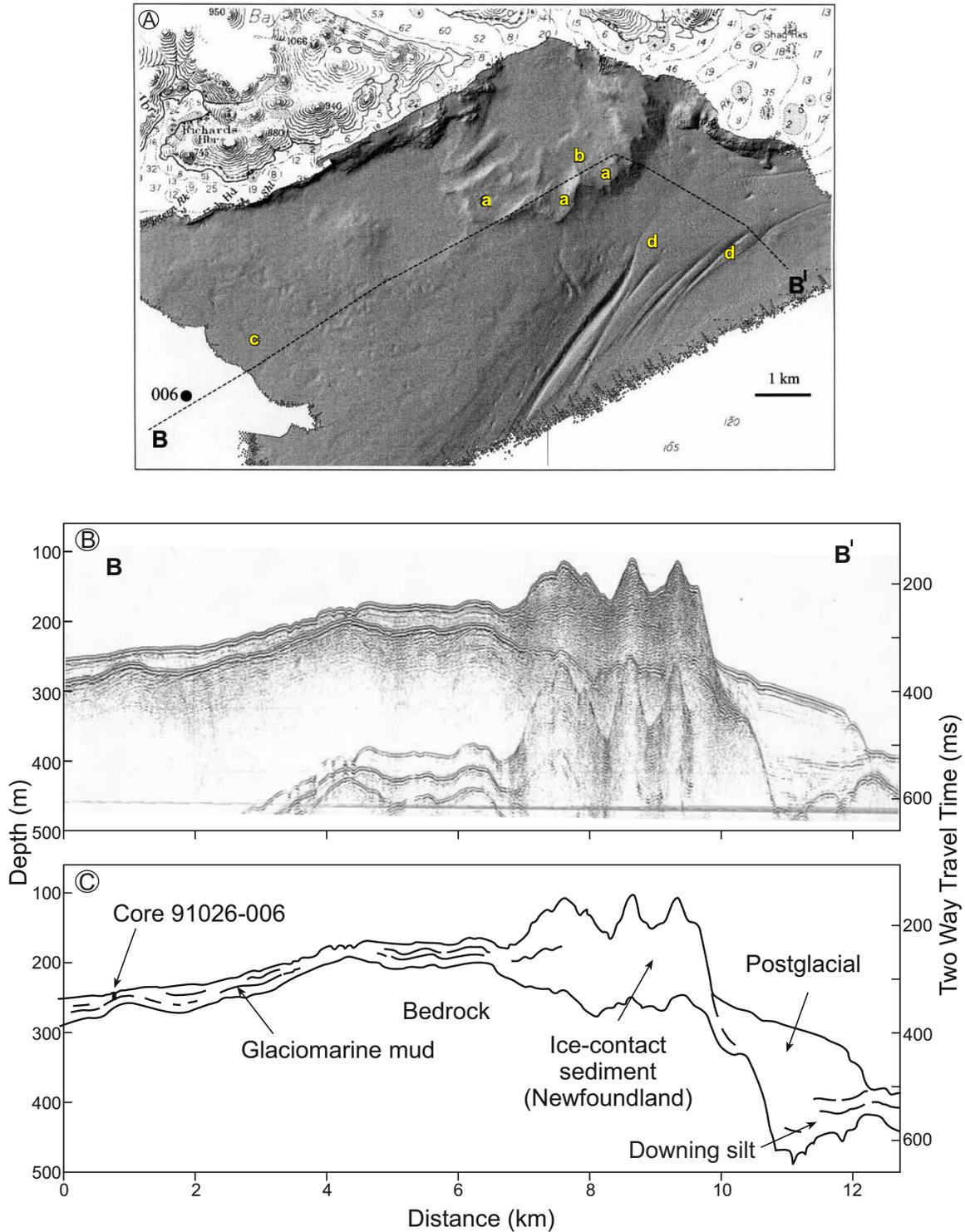
**Figure 4.** A) Shaded-relief multibeam image of the submarine moraine off Facheux Bay, which has convex-seaward ramps (a) and prominent landward cusps (b), iceberg furrows and pits (c) and long, deep arcuate iceberg furrows (d). B-B' is line of the sleeve-gun record taken over the moraine; B) Sleeve-gun record across the submarine ridge off Facheux Bay; C) Interpretation showing the location of the ice-contact sediment. All illustrations taken from Shaw et al. (2000).
