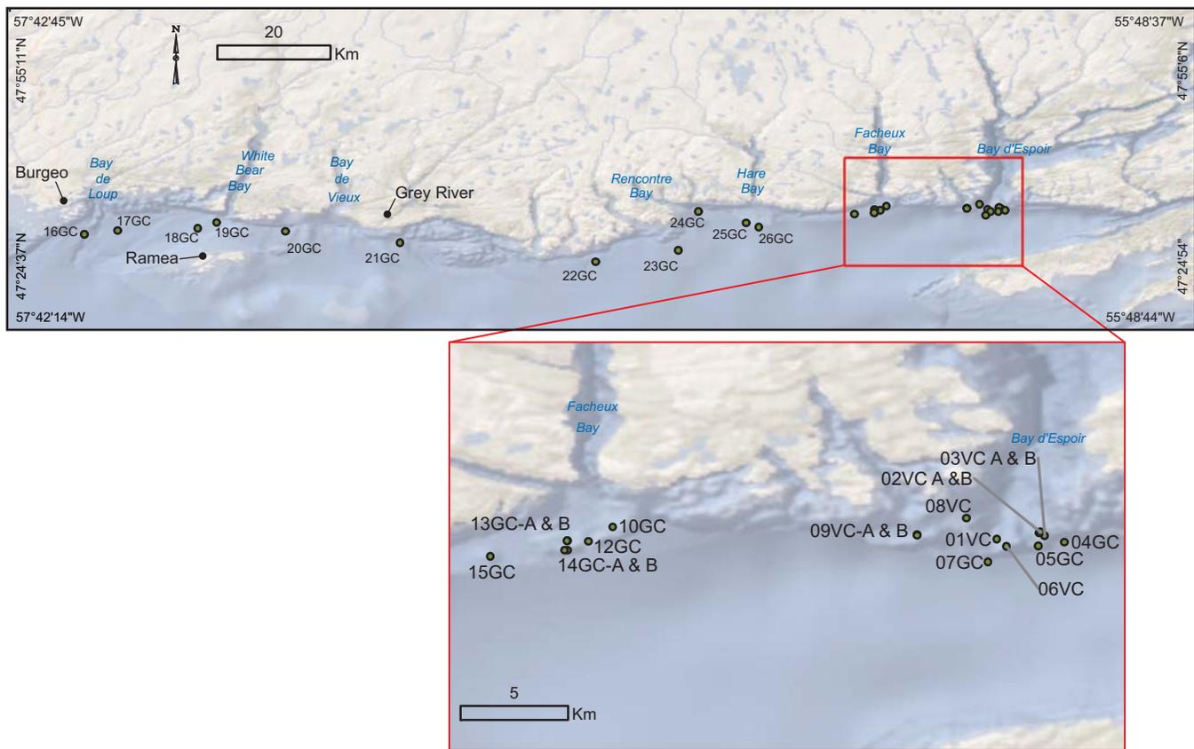
**Figure 6.** Location of coring stations between Bay d'Espoir and Burgeo. Black dots show locations of neighbouring communities. Inset shows enlarged area of Facheux Bay and Bay d'Espoir. The letters after the site numbers refer to the type of corer used: GC – gravity corer; VC – vibro-corer.
