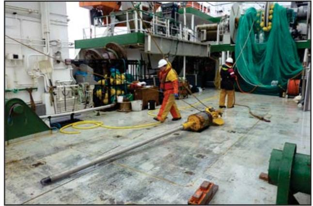
**Plate 2.** Gravity corer used during the NISS survey.
