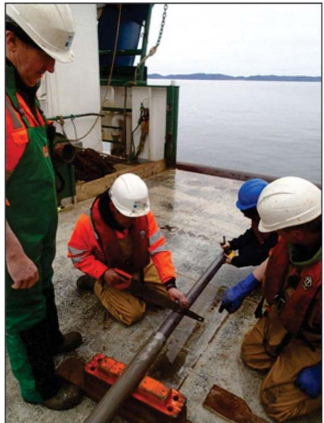
**Plate 3.** Core liner was measured into 1 m segments and cut with a handsaw. Caps were placed on the ends of the core after cutting.
