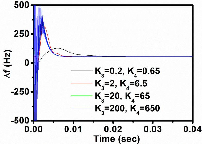
Figure 4. Transient and steady state behaviour of frequency shift for different controller gains. The simulation parameters are:  $R = 3 \text{ (nm)}$ ,  $k = 4 \frac{\text{N}}{\text{m}}$ ,  $Q = 240$ ,  $H = 5 \times 10^{-20} \text{ (J)}$ ,  $E = 100 \text{ MPa}$ ,  $A = 10 \text{ (nm)}$  and  $z_c = 9.5 \text{ (nm)}$ ,  $f_0 = 156.719 \text{ kHz}$ .
