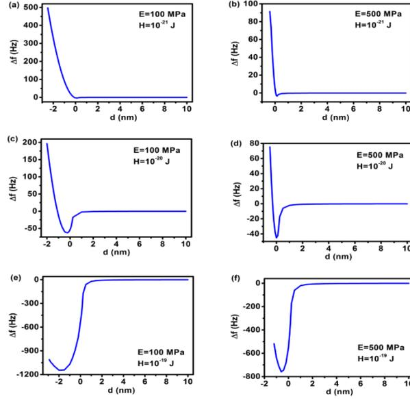
Figure 5. Frequency response of FM-AFM for different samples with different stiffness and Hamaker constant.
