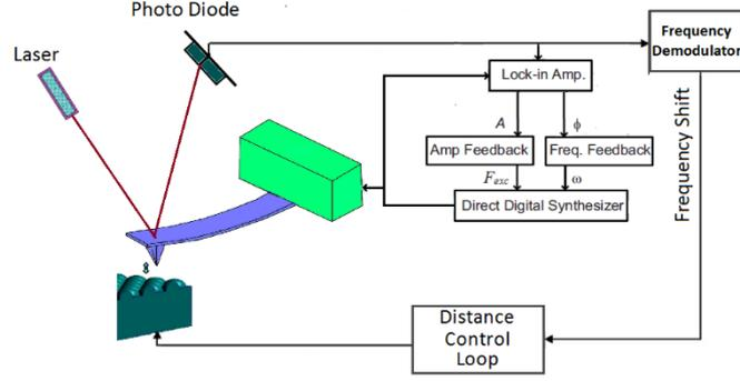
Figure 1. Schematic representation of FM-AFM.
