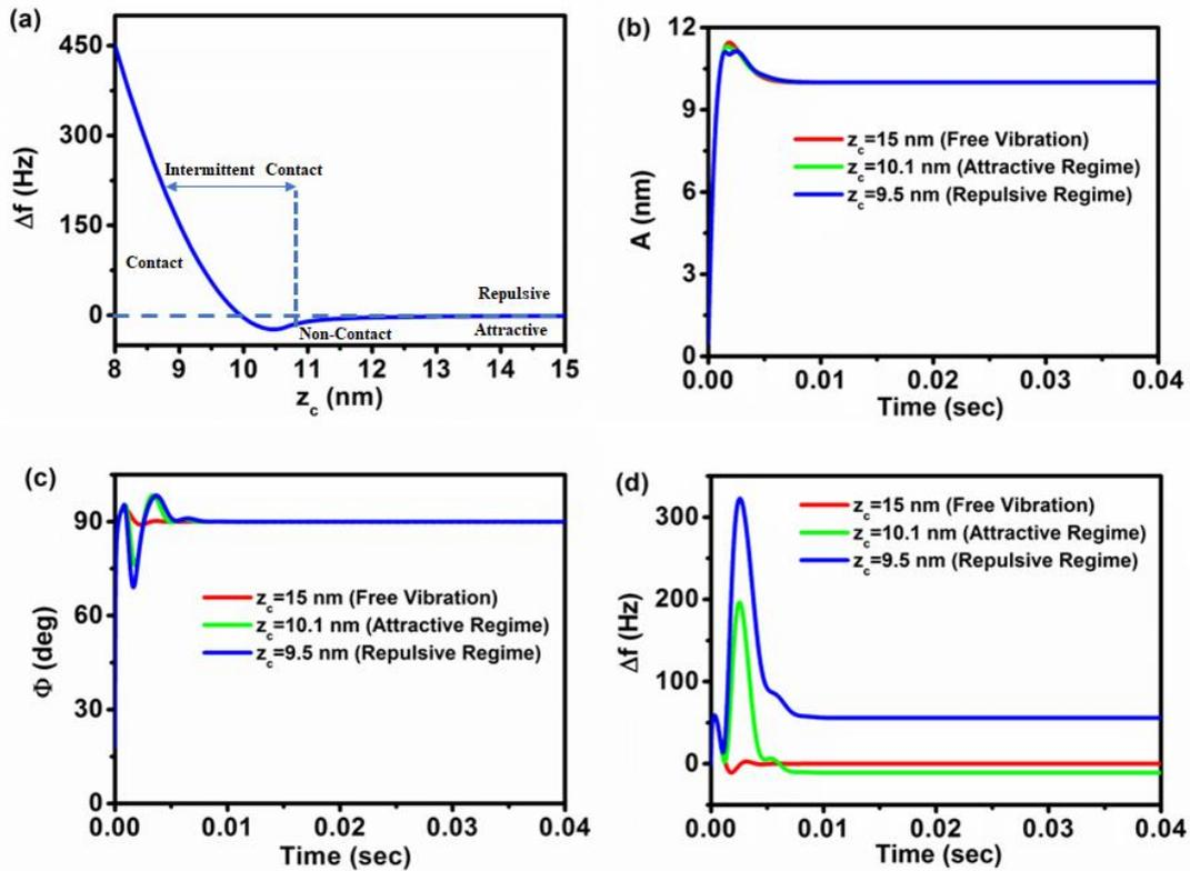
Figure 3. a) Frequency shift versus average distance, transient and steady state response of b) amplitude, c) phase and d) frequency shift of cantilever. The simulation parameters are:  $R = 3$  (nm),  $k = 4 \frac{N}{m}$ ,  $Q = 240$ ,  $H = 5 \times 10^{-20}$  (J),  $E_{eff} = 100$  MPa,  $E_s = 85$  MPa,  $v_s = 0.4$ ,  $A = 10$  (nm),  $a_0 = 0.164$  nm.
