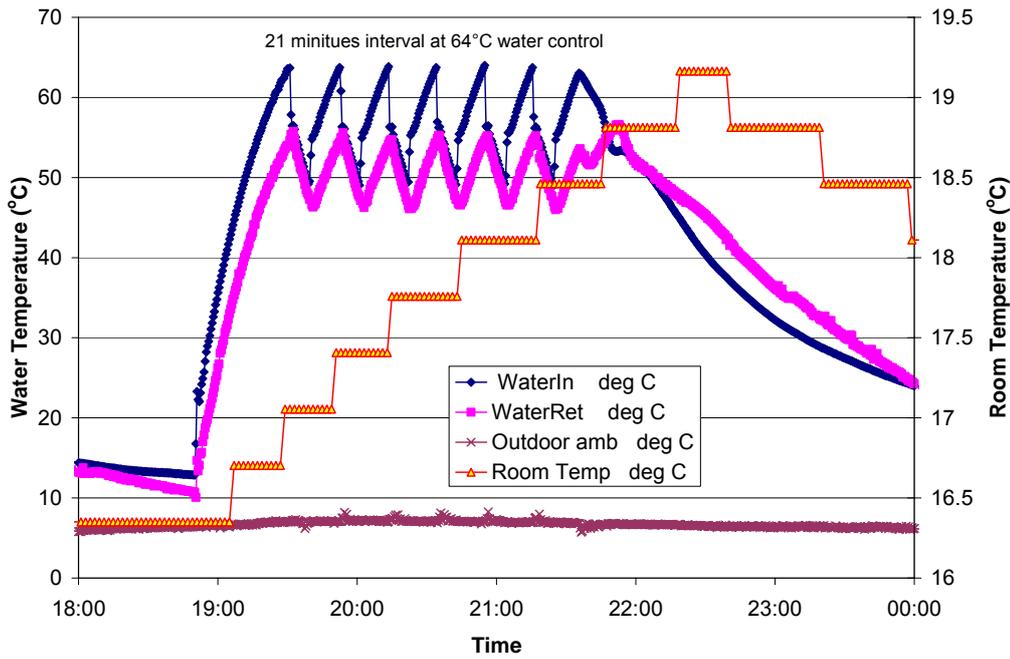
Figure 2 Temperatures of on-off control HP system with indoor and outdoor ambient temperature
