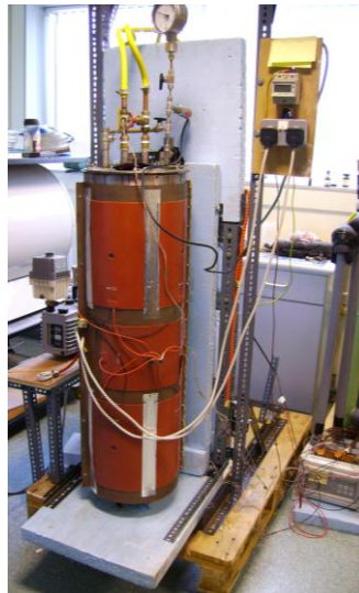
152 153 154 155 156 157 158 159 160 161 162 163 164 165 166 Figure 5: Images of the Mark IV unit under heat flux simulator test conditions
