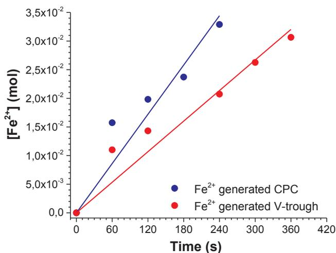
Fig. 3. Fe<sup>2+</sup> generation for CPC and V-trough reactors during actinometrical test.
