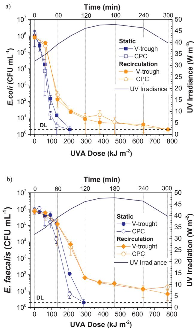
Fig. 4. Solar inactivation of *E. coli* (a) and *E. faecalis* (b) in isotonic water within CPC and V-trough solar reactors in recirculation and static modes.
