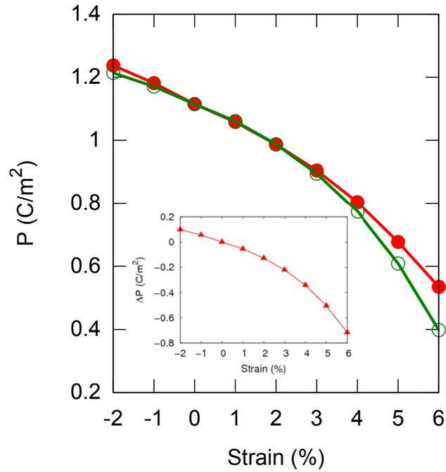
Figure 3: The total spontaneous polarization ( $P$ ) along the  $c$ -direction as a function of epitaxial strain. Red filled circles represent directly calculated values using Eq. (1), and green open circles represent values estimated using Eq. (2).  $\Delta P$ , which is the change in spontaneous polarization along the  $c$ -direction due to the epitaxial strain, as a function of epitaxial strain is shown in the inset.
