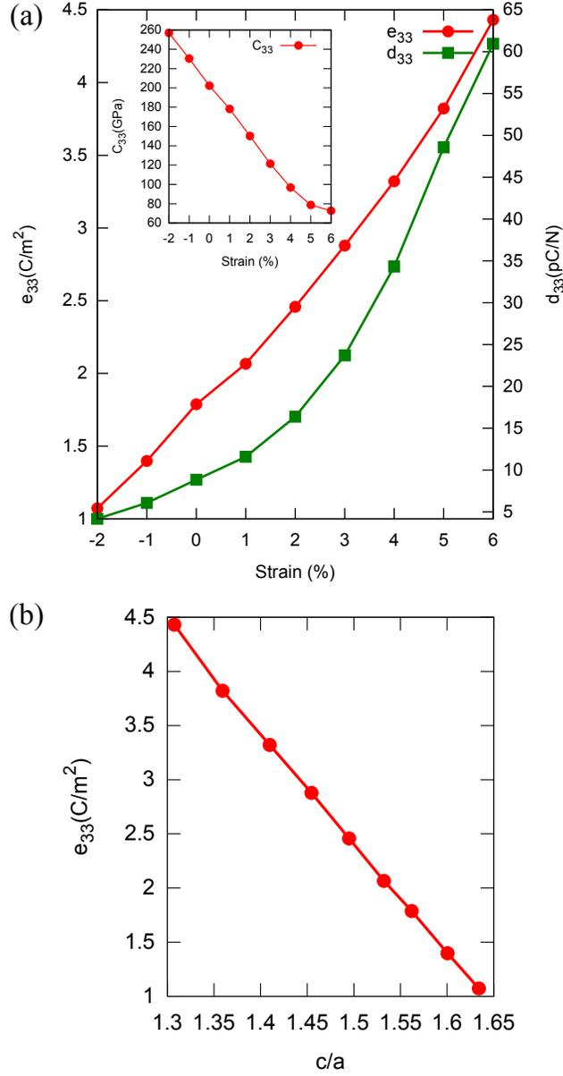
Figure 4: (a) Change in piezoelectric constants ( $e_{33}$  and  $d_{33}$ ) with epitaxial strain. Inset shows the change in elastic constant  $C_{33}$  with epitaxial strain. (b)  $e_{33}$  as a function of the  $c/a$  ratio as the  $c/a$  ratio changes due to the epitaxial strain.
