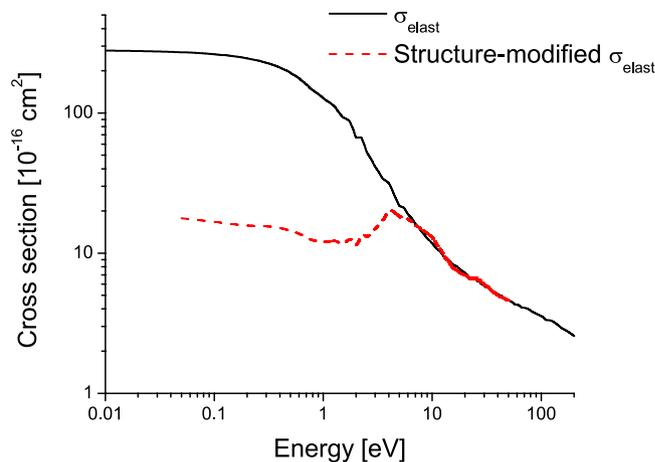
**Figure 3. Impact of coherent scattering effects on the elastic momentum transfer cross-section for positron-water scattering.** The static structure factor for water used in presented in Fig. 4<sup>26</sup>.
