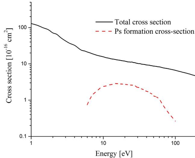
**Figure 2. The total and Ps-formation cross-sections for positrons in water vapour.** The full details of the cross-section used are detailed in<sup>21–25</sup>.
